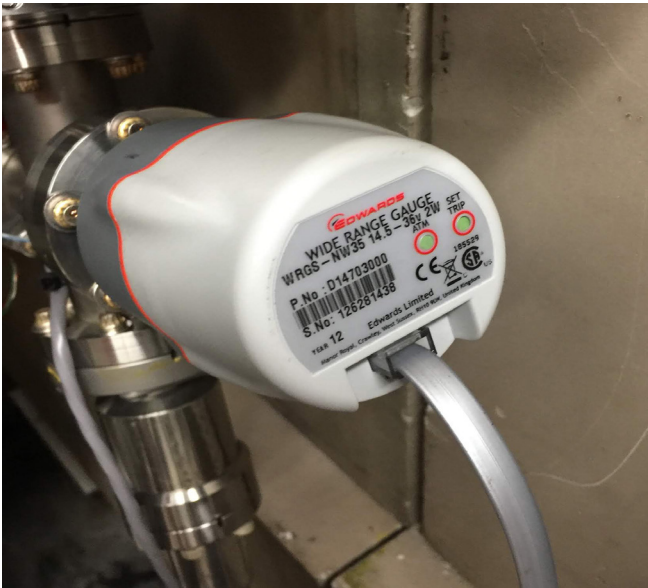
FIG. 1. Edwards WRG installed on Hall C HMS spectrometer.
